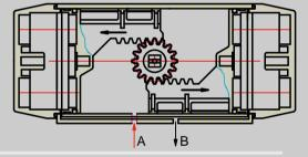
Air to Port A forces the pistons outwards, causing the pinion to turn counterclockwise while the air is being exhausted from Port B.  $\ensuremath{\mathsf{CCW}}$
