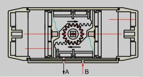
Air to Port B forces the pistons inwards, causing the pinion to turn clockwise while the air is being exhausted from Port A. CW
