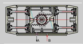
Loss of air pressure, the stored energy in the springs forces the pistons inwards, the pinion turns clockwise while air is being exhausted from Port A.
