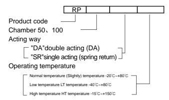
Description: Actuator Mode RP50, Type Double Acting and low temperature
